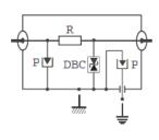
P: Spark Gap DBC: Clamping Diod R: Resistor
